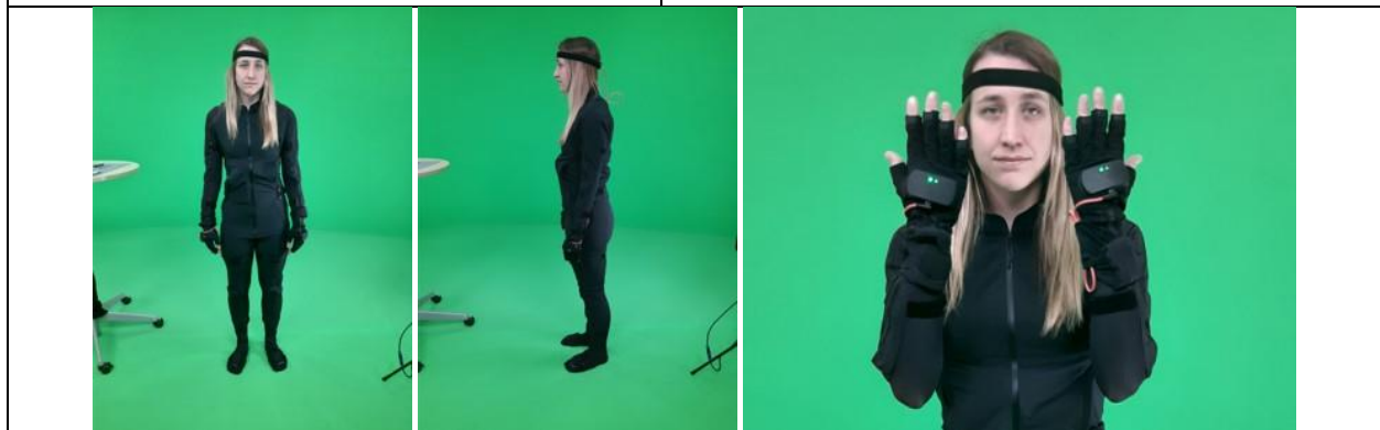
Figure 4- All-in-one motion capture solution using the Smartsuit Pro II and Smartgloves. The whole-body movements were recorded, including the hands' gestures. All components are portable, allowing the expert to perform gestures as they would in a real medical environment.
